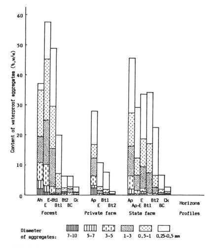
Fig. 1. Water stability of soil aggregates.
